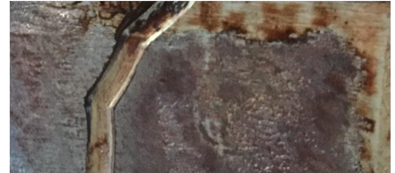
Trace pollution of 0.1% PVC in PP causing corrosion of a steel mold for PP. © MGG Polymers
