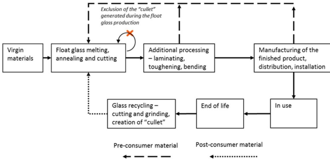
Figure 4 : Schematic diagram to distinguish pre-consumer and post-consumer recycled material in glass
